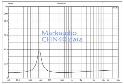
FS 97.4826 Hz VAS 1.1523 L RE 6.8000 Ohm QMS 3.7689 QES 0.7752 QTS 0.6429 Bxl 3.1071 Txm SPL 83.41 SD 0.0023 m2 CMS 1.5733 mm/N MMS 1.6942 g RMS 0.2753 WM RAT 307716 WA RMT 1.6140 WM MMD 1.6322 g 0.13% h0 L1kHz1.0575 mH PWR 7 watts (Nom) X MAX (Mech) +/- 3.5mm
